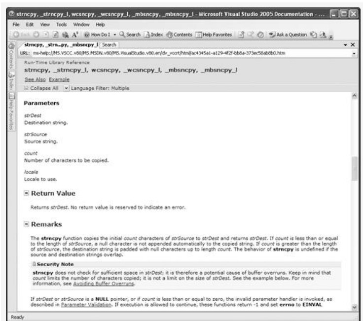
Figure 10-2. Developer documentation for the C runtime strncpy function, drawing the developer's attention to security issues when using the function.
