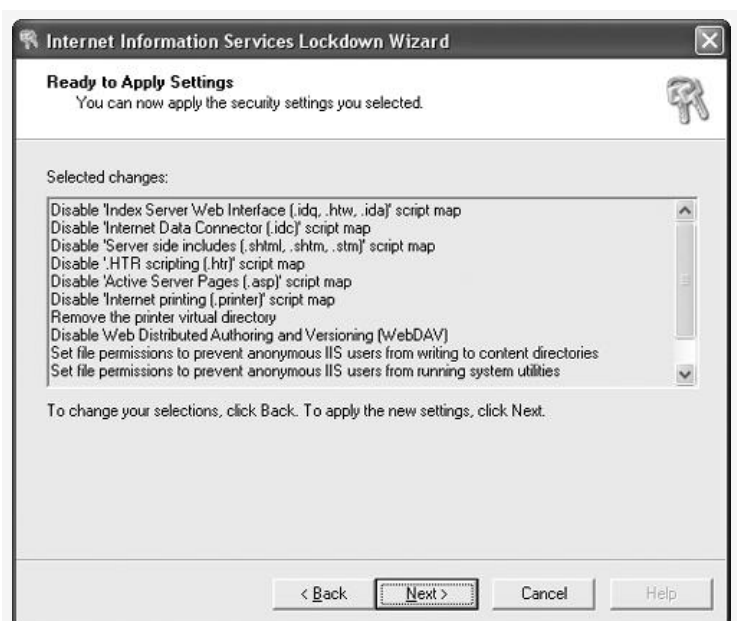
Figure 10-1. The IIS Lockdown tool about to lock down ("harden") an IIS 5.1 server on Windows XP Service Pack 2 (SP2).
